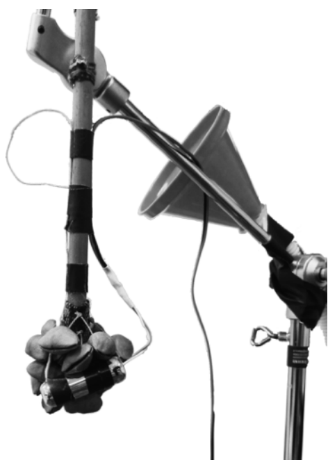
Vibrator 1: attached below/inside small rattler. The rattler should sound (continuous noise) when vibrator is on.
