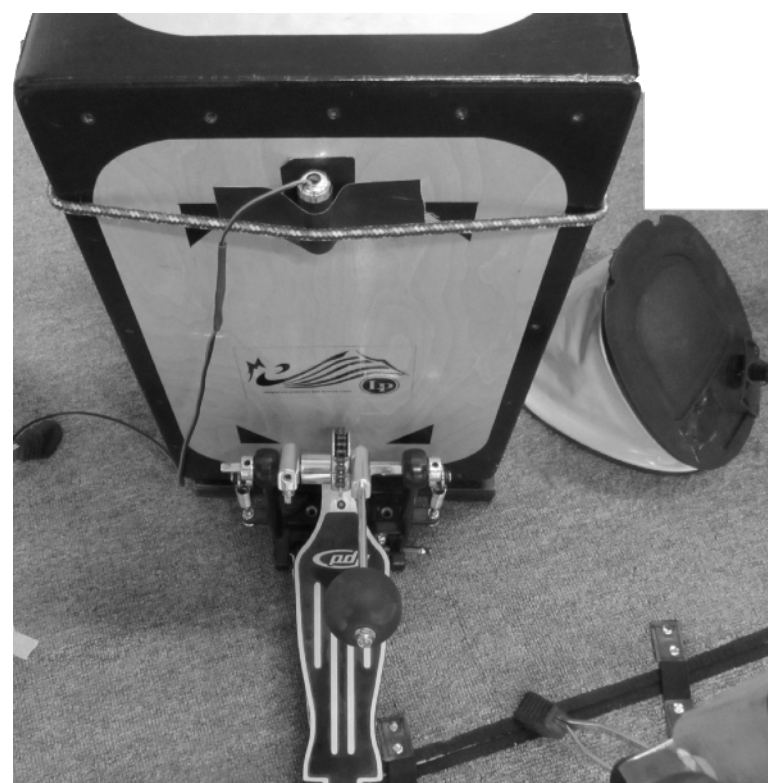
Vibrator 6: attached on cajon with duct tape and rubber strap to make a low pitch with a small amount of distortion.
